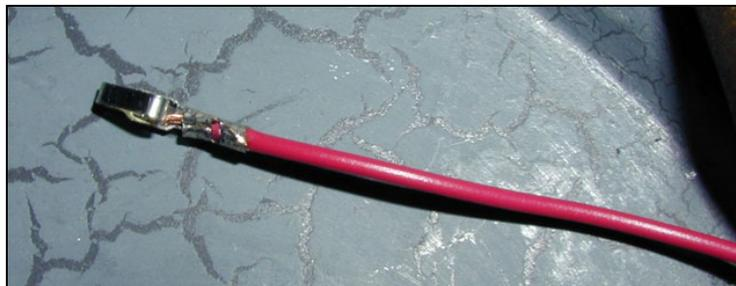
To install into the plug housing, I aligned the small locking tab (near the base) on the connector with the retaining clip in the housing and inserted. They will push all the way through if you go too far, however you'll know it's far enough when the connectors click and you can't pull them back out the way they came in. If they don't retain, they're in upside down.
