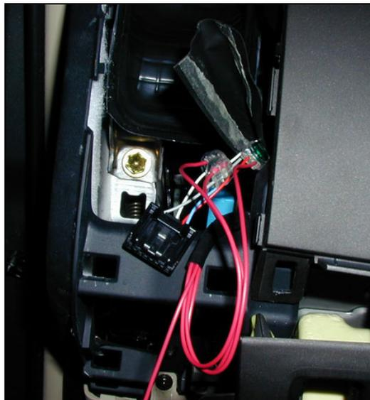
After that, I tested the EV button illumination by plugging in the dimmer to the plug, and turning on the parking lights. Success should yield an illuminated EV button which is brightness adjustable.
