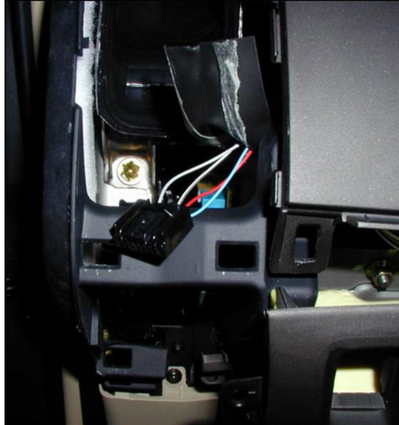
After trimming the 3 short leads to a reasonable size, using green Radio Shack Telephone taps (RS part number 64-3081, I tapped the IL(+) lead - pin 1 - to the grey wire from the dimmer harness, the IL(-) lead - pin 2 - to the red wire from the dimmer harness, and the EV(-) - pin 4 - to the white/black stripe wire from the dimmer harness. I then taped the wires together, and then closed the rubber coating as best as I could, using electrical tape to hold it together.
